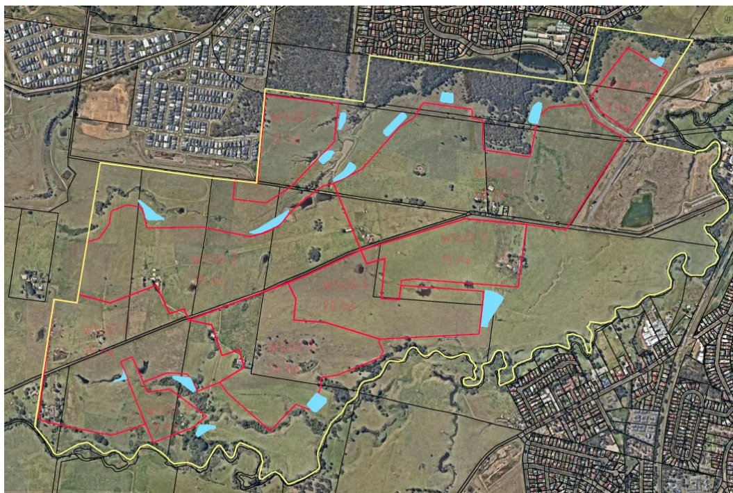
Figure 19 Post development catchment plan for WSUD Measures (Rienco)
